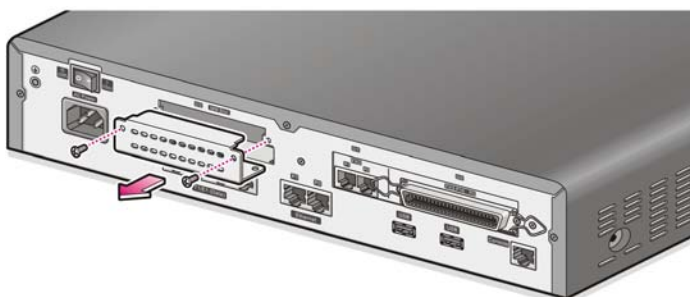
Figure 5.7 Preparing a mini-module slot for module insertion
