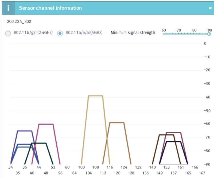
**Figure 85. Channels information-802.11a/n/ac (5 GHz)**
