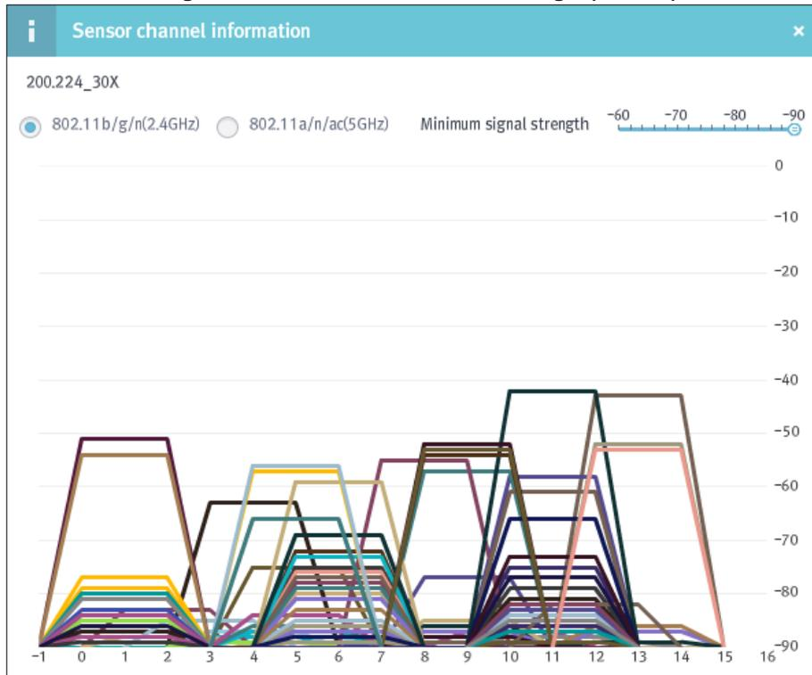
The signal intensity and the information on channels by the SSID detected in the bandwidth at 2.4 GHz are displayed; by adjusting or moving the slider for **the minimum value of signal intensity (dBm)**, you may selectively view only the information on the SSID having the predefined value or higher.
