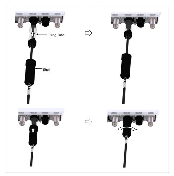
Figure 47. Connecting the PoE Cable (3)
