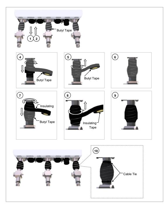
Figure 55. Connecting the Arrestors (3)
