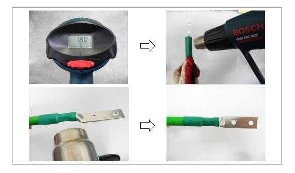
Figure 89. Assembling Heat Shrink Tube (2)
