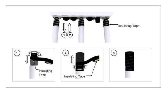
Figure 8. Assembling the Dipole Antennas (2)
