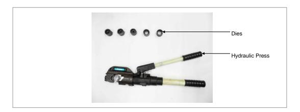
Figure 83. Fixing Pressure Terminal\_Hydraulic Press (1)
