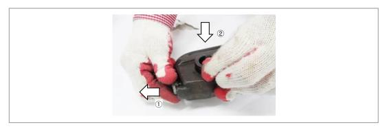
Figure 84. Fixing Pressure Terminal\_Hydraulic Press (2)
