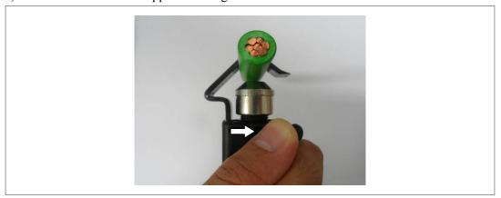
Figure 75. Stripping Cable Sheath (4)
