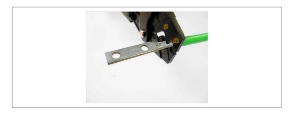
Figure 81. Fixing Pressure Terminal\_Handheld Compressor (4)
