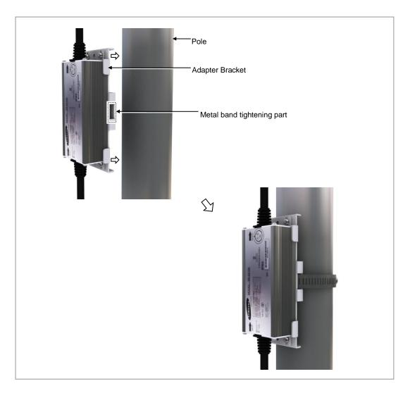
Figure 26. Mounting the Adapter on a Pole (2)
