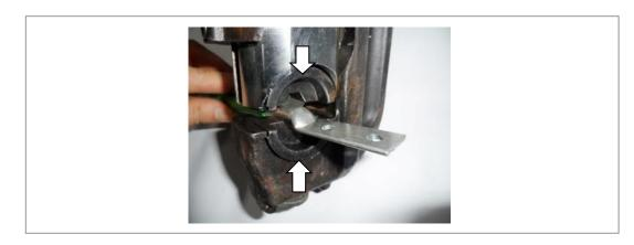
Figure 85. Fixing Pressure Terminal\_Hydraulic Press (3)
