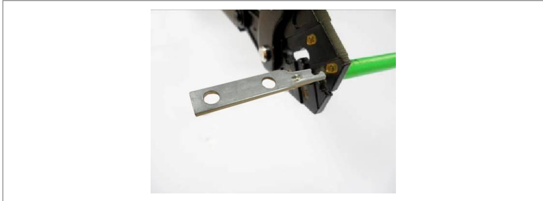
Figure 81. Fixing Pressure Terminal_Handheld Compressor (4)
