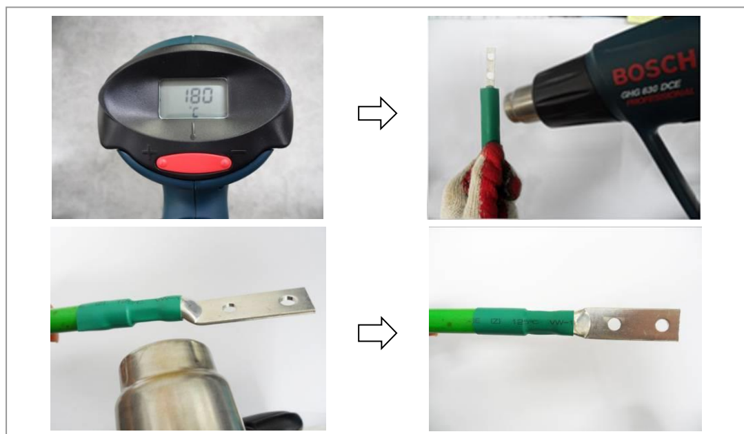
Figure 89. Assembling Heat Shrink Tube (2)
