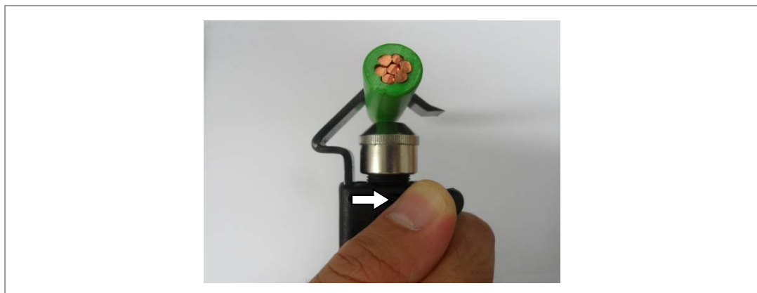
Figure 75. Stripping Cable Sheath (4)
