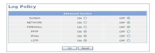
Select added logs from the logs for system log, network, firewall, VPN, and click the **[OK]** button to add logs to the system log. Click the **[Reset]** button to return to the previous status before applying the configuration.
