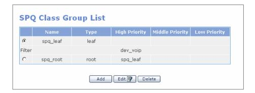
Click the [Add] button of the SPQ Class Group list in the <Class Group> window. Then, the window that can set SPQ class group appears. If Class Type is set to leaf, the window displayed is as follows. Set the ID and filter of leaf class and click the [OK] button.
