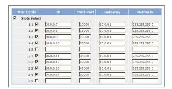
Up to ten MGI cards can be entered into this table. The figures on the left side indicate the locations of the cabinet-slots. The 'Start Port' means the number of the first port among the 32 external ports where the services are to be provided in the MGI card. If there is no entered number, the setup is autumatically made as the values increasing by 5000 from no. 1000 as the orders of the cabinets or slots.
