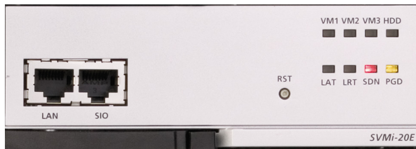
Figure 3.50 SVMi-20E LED Indications
