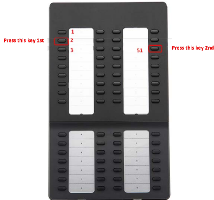
Figure 7.29 Setting-Up SMT-i5264 AOM
