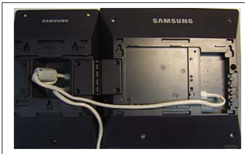
Figure 7.28 Attaching SMT-i5264 AOM to phone
