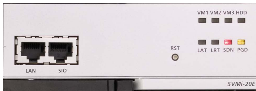
Figure 3.50 SVMi-20E LED Indications
