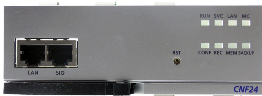
Figure 3.53 CNF24 LED Indications
