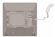
OPTIONAL: Connect the cable through the middle hole of the cradle to the PC, as shown in the figure. When connecting to PC, connect one end of the cable to the PC port of the phone, and the other end of the cable to the LAN port of the PC.
