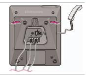
Secure the cable along the cable guideline as shown in the figure. For the cable of power adaptor, give some slack before securing the cable to the guideline to prevent easy disconnect.
