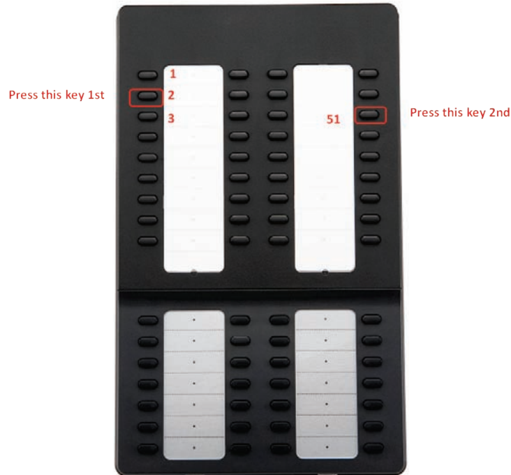
Figure 7.20 Setting-Up SMT-i5264 AOM
