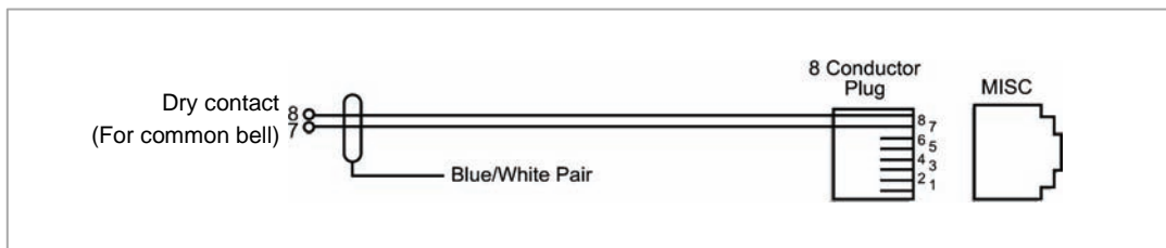
Figure 7.26 Connecting Common Bells
