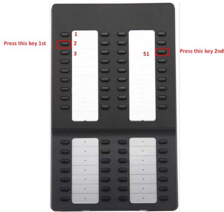
Figure 7.20 Setting-Up SMT-i5264 AOM
