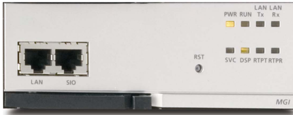
Figure 3.43 Front View of the MGI Board
