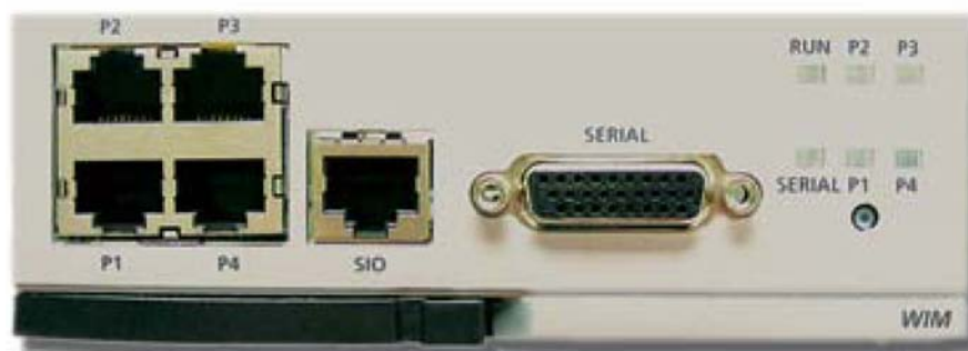
Figure 3.34 Front View of the WIM Board
