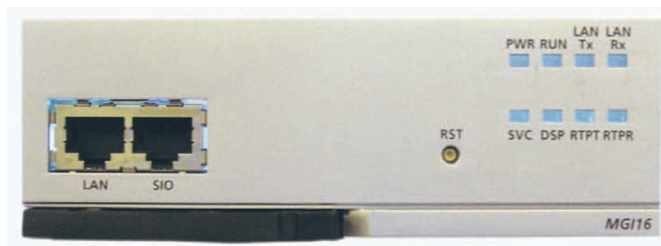
Figure 3.44 Front View of the MGI-16 Board
