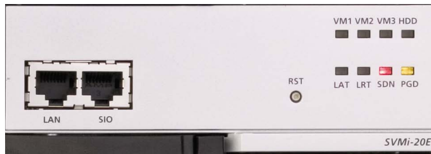
Figure 3.49 SVMi-20E LED Indications
