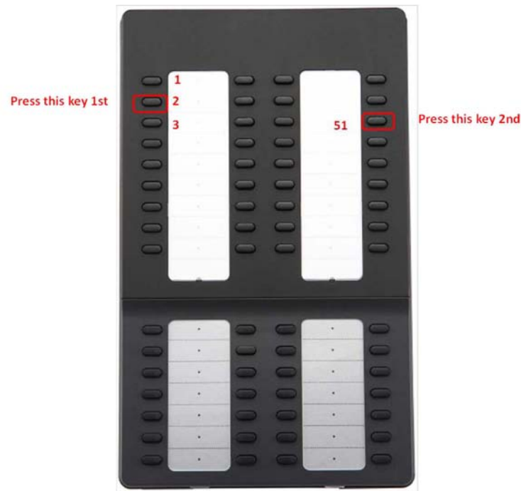
Figure 7.30 Setting-Up SMT-i5264 AOM
