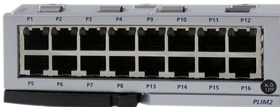
Figure 3.38 Front View of the PLIM2 Board
