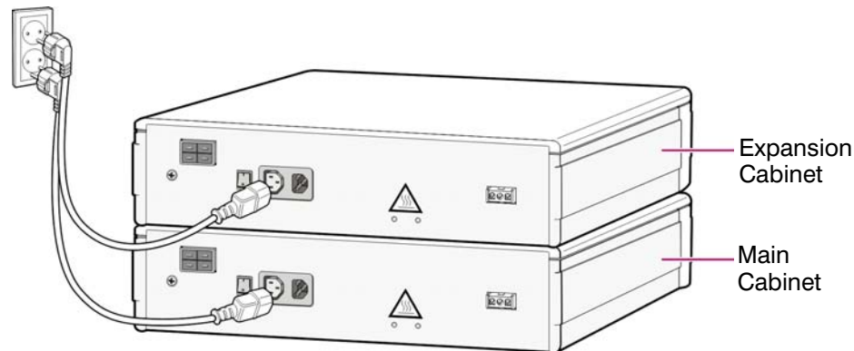
Figure 5.2 Connecting Power (using Power Cable)
