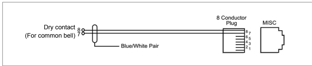
Figure 7.23 Connecting Common Bells
