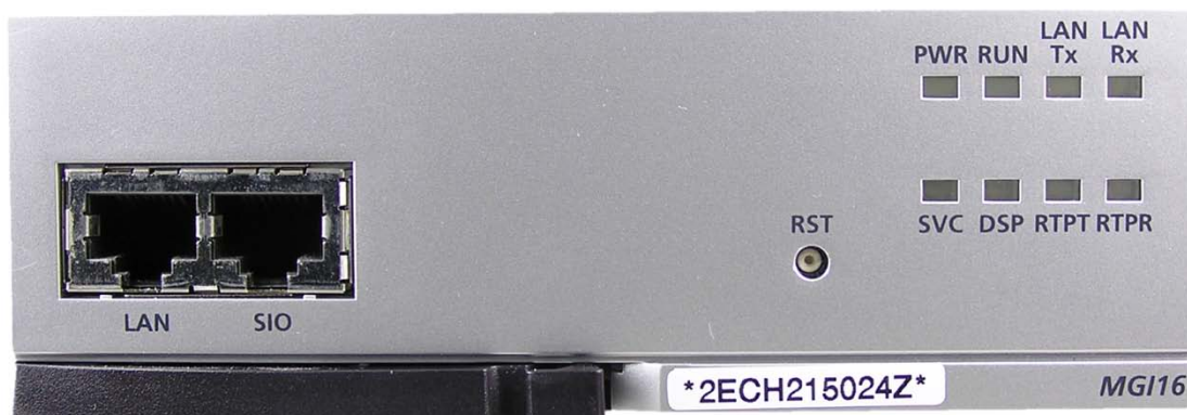
Figure 3.32 Front View of the MGI16 Card
