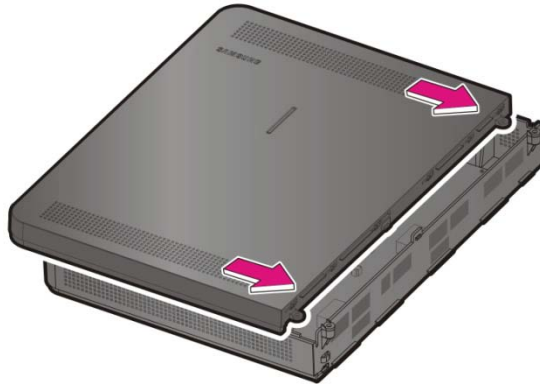
Figure 2.13 Installing the top cover (1)
