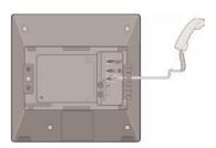
OPTIONAL: Connect the cable through the middle hole of the base to the PC, as shown in the figure. When connecting to PC, connect one end of the cable to the PC port of the phone, and the other end of the cable to the LAN port of the PC.
