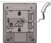
OPTIONAL: Connect the cable through the middle hole of the base to the PC, as shown in the figure. When connecting to PC, connect one end of the cable to the PC port of the phone, and the other end of the cable to the LAN port of the PC.
