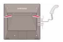
Secure the cable along the cable guideline as shown in the figure. For the cable of power adaptor, give some slack before securing the cable to the guideline to prevent easy disconnect.
