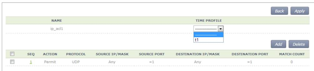
Figure 31. Window where a Time Profile is Applied to ACL
