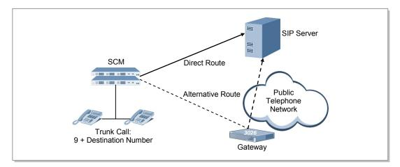
Figure 22. Making a trunk call via SCM
