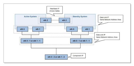
Figure 44. Redundant System IP Address Configuration
