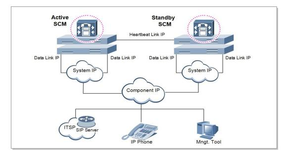
The following diagram shows the redundancy structure of SCM.
