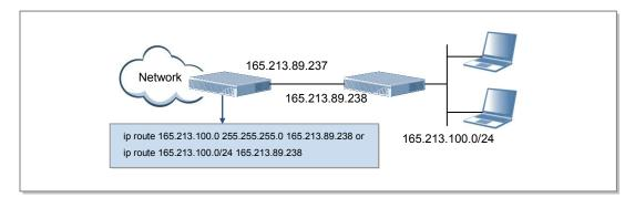
Figure 31. Simple network configuration for static route
