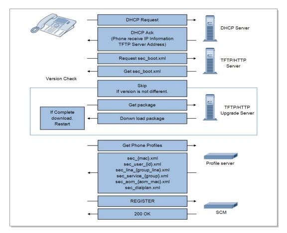
Figure 29. Automatic Upgrade Procedure
