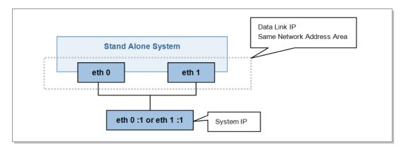
Figure 43. Standalone System IP Configuration
