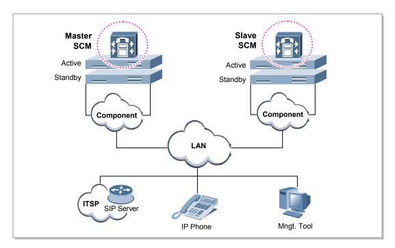
Figure 45. Active-Active and Geo-Redundancy
