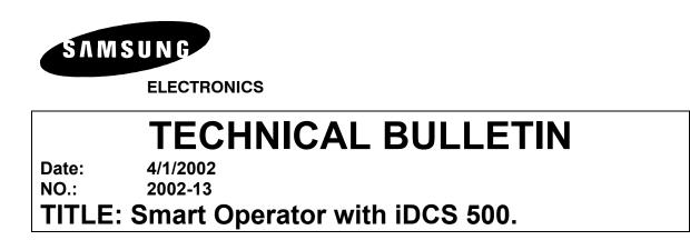
The purpose of this bulletin is to inform the dealer of a problem that may occur on the iDCS 500 when using Smart Operator. If there is a Trunk card (TEPRI, TRKC1, TRKB1) installed in the first slot, the Smart Operator will not function. This has been corrected in the Smart Operator software Version 1.2.
