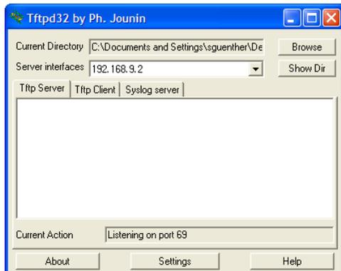
6. The TFTP server is now configured and ready to receive update requests. Make note of the IP address displayed in the "Server interfaces" text box.
