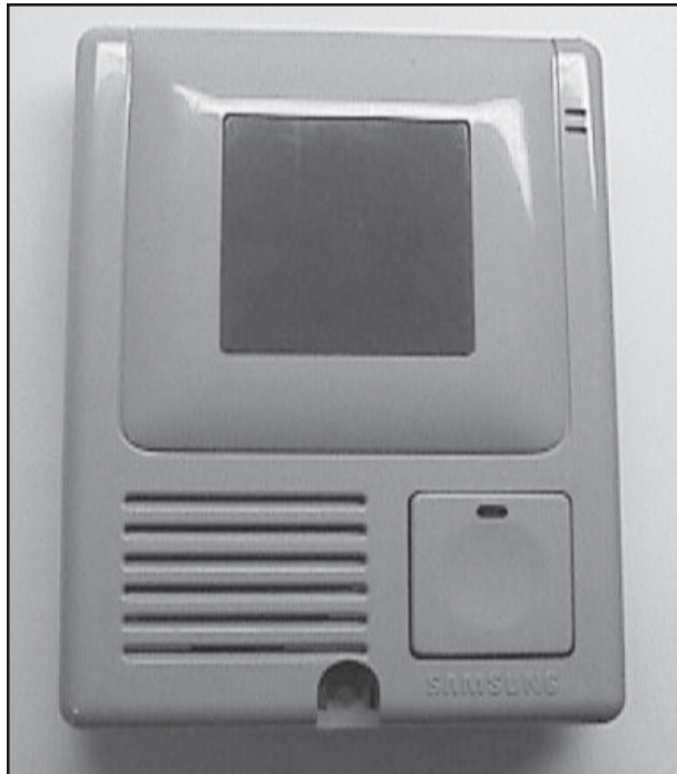
Figure 3. UDPH (Universal Doorphone Unit)
