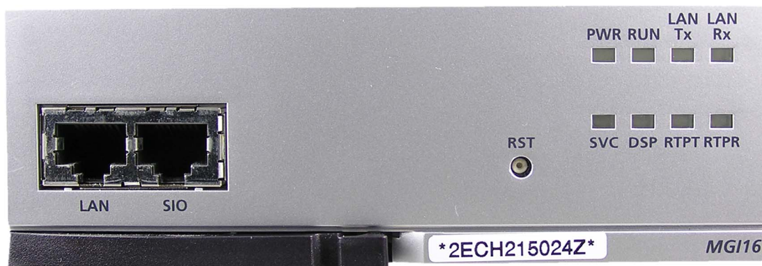
Figure 3.28 Front View of the MGI16 Card
