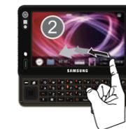
**Note:** Tapping or touching individual entries on the list opens the list entry. Scrolling requires that you press firmly on the screen then drag. When scrolling through a list (see adjacent image) make sure not to touch or press individual entries on the list as this will open the list entry.
