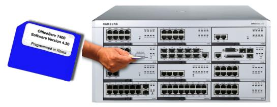
Beginning with the launch of new system software V4.30i all software for the OfficeServ 7400 will be delivered on an SD media card. The SD Media card comes with a write protect switch. This switch must always be in the unlocked position which the switch is towards the electrical leads.
