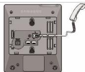
OPTIONAL: Connect the cable through the middle hole of the base to the PC, as shown in the figure. When connecting to PC, connect one end of the cable to the PC port of the phone, and the other end of the cable to the LAN port of the PC.
