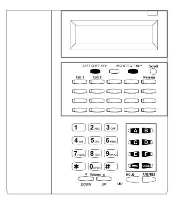
This diagram illustrates the keys on a **iDCS 8 BUTTON keyset** that have special functions during programming. When required, these keys will be referred to by the names described in the diagram.
