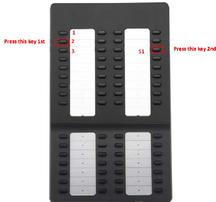
Figure 7.29 Setting-Up SMT-i5264 AOM
