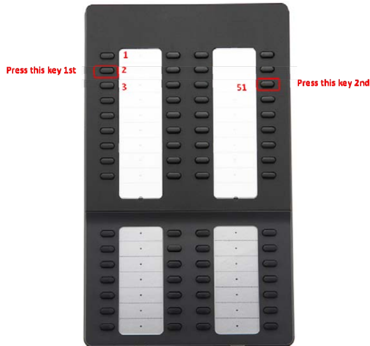
Figure 7.30 Setting-Up SMT-i5264 AOM
