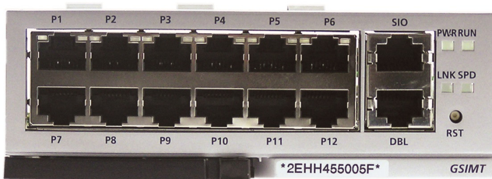
Figure 3.41 Front View of the GSIMT
