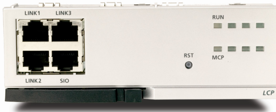
Figure 3.9 Front View of the LCP
