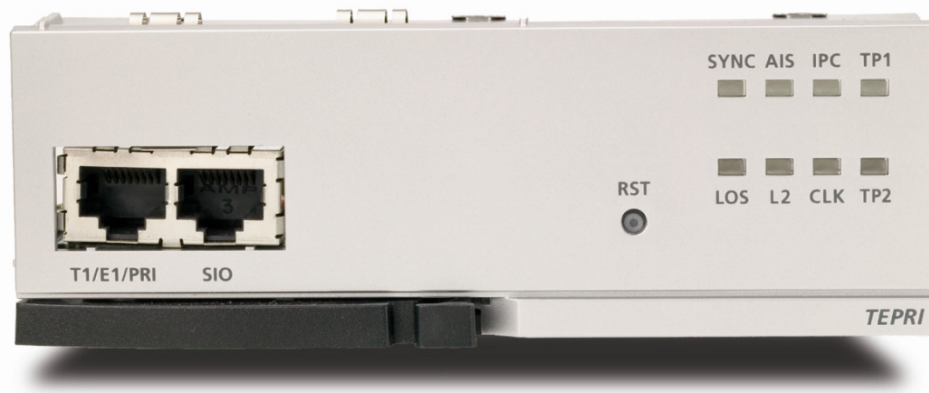
Figure 3.20 Front View of the TEPRI
