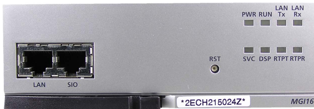
Figure 3.32 Front View of the MGI16 Card
