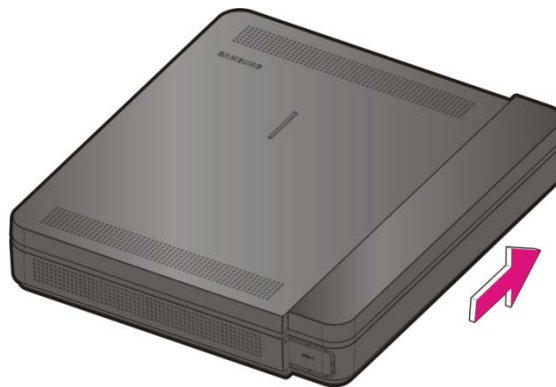
Figure 2.1 Removing the cable duct cover (1)
