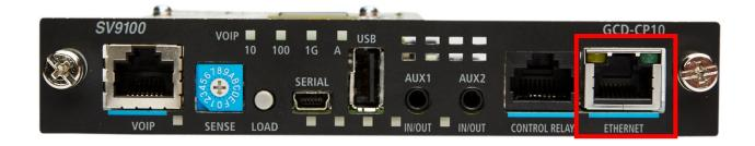
If the CPU has a VoIPDB (GPZ-IPLE) installed, the default IP Address for the **VOIP** connection is **172.16.0.10**
