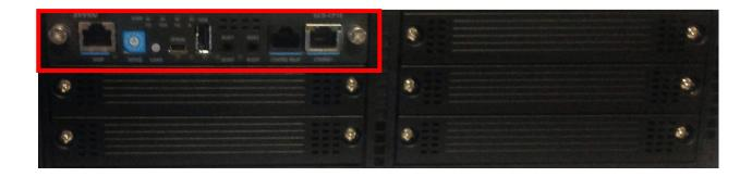
Press and hold the LOAD button while you turn on the power button.
