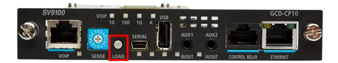
The LED below and to the right of the SERIAL connection will turn solid red.
