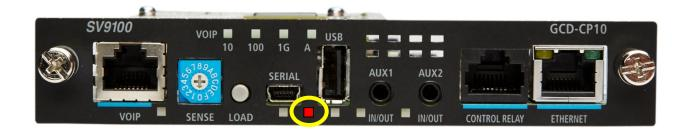
Continue to hold the Load button until the 3<sup>rd</sup> LED turns solid red.
