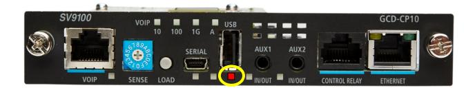
When that happens, release the LOAD button and wait until the CPU RUN LED flashes Green.
