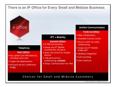
IP Office editions allow a customer to match a solution to their specific requirements. Basic Edition provides key system and PBX features. Each subsequent edition provides increasing levels of features and sophistication.
