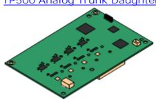
This card allows the base card to support 4 analog loop-start trunks.
