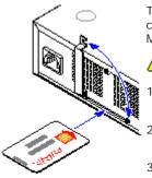
The IP500 uses a smart card feature key dongle. In addition to feature licensing the IP500 control unit uses this feature key dongle to determine various systems defaults such as A-Law or Mu-Law operation, default short codes and trunk settings.
