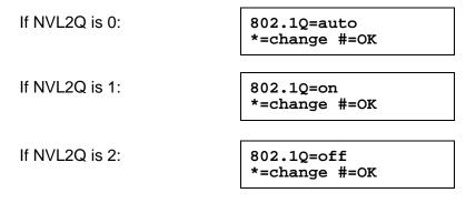
7. Press \* to change **802.1Q** to the next sequential value. For example, if the current value is 0 (auto) pressing \* changes it to 1 (on) and if the current value is 2 (off), pressing \* changes it to 0 (auto).
