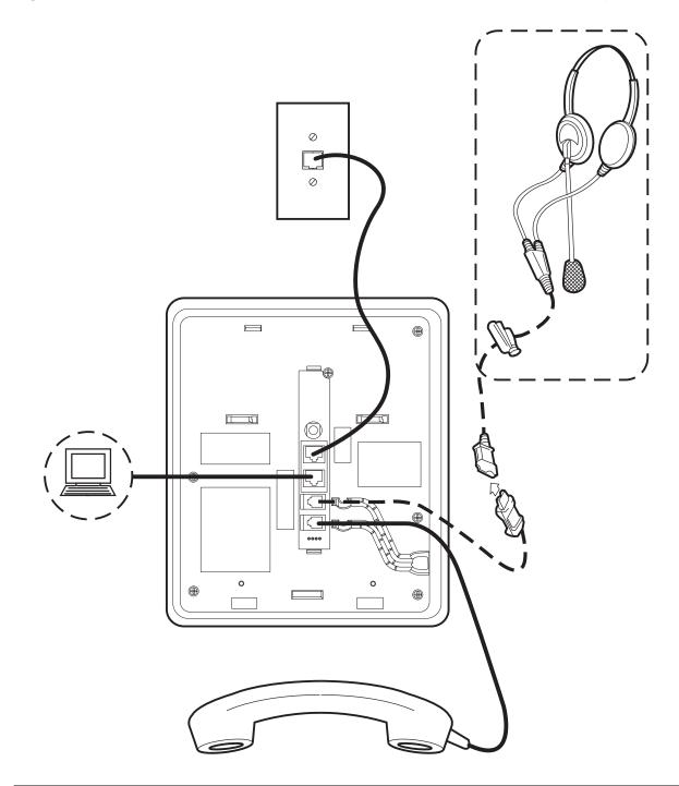
Figure 3: Connection Jacks with Power over Ethernet on a 1608 Series IP Telephone
