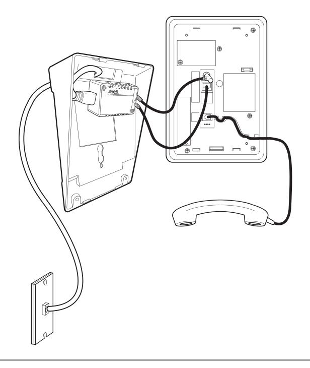
Figure 1: Connection Jacks with Power over Ethernet on a 1603 Series IP Telephone
