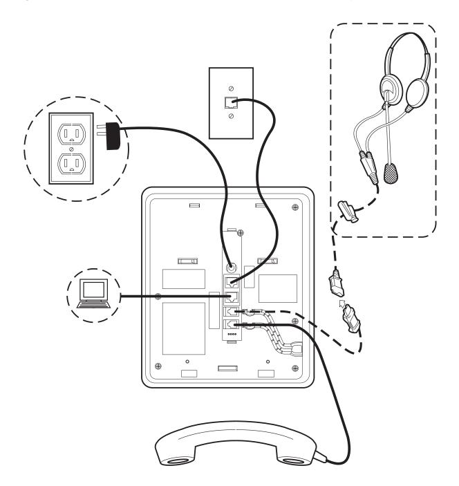
Figure 4: Connection Jacks with Local Power on a 1608 Series IP Telephone
