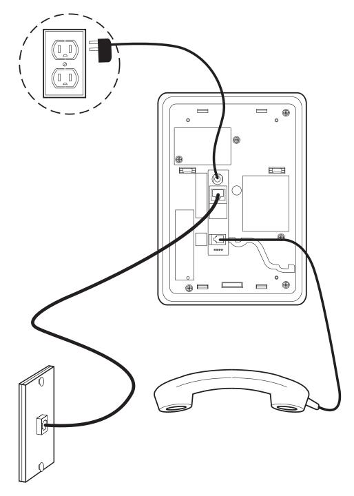
Figure 2: Connection Jacks with Local Power on a 1603 Series IP Telephone
