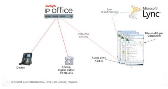
Figure 1: Avaya Lync Integration deployed in an Enterprise
